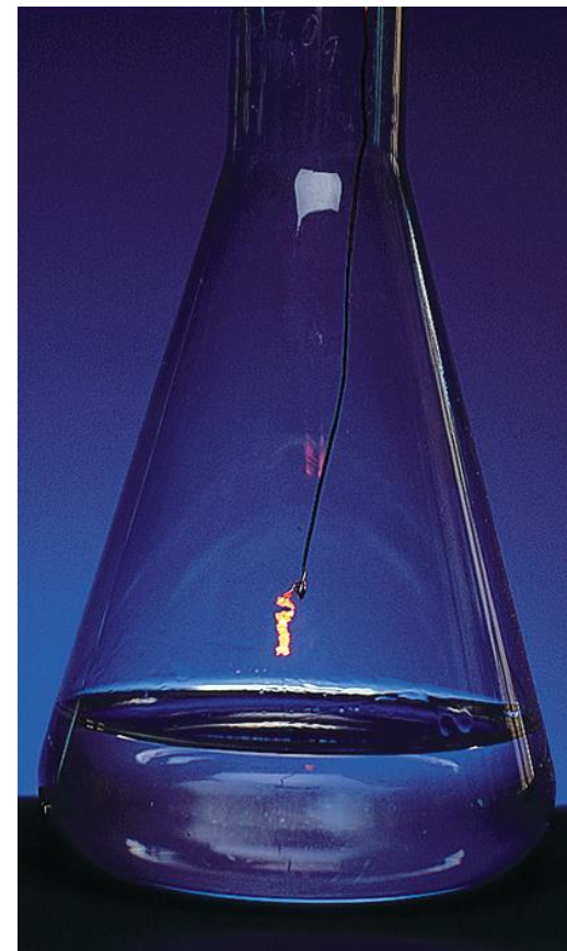
Hot Pt wire over \text{NH}_3 solution
